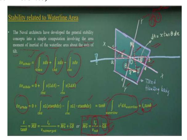
Now how to compute this the metacentric height? Let you have a floating object like this, okay? And you consider the unit width of this ones which is a perpendicular to this surface that is what unit width is there. So what we will do it let have the initial positions of waterlines goes through this C to D. So initially it was C to D and it was tilted okay.
