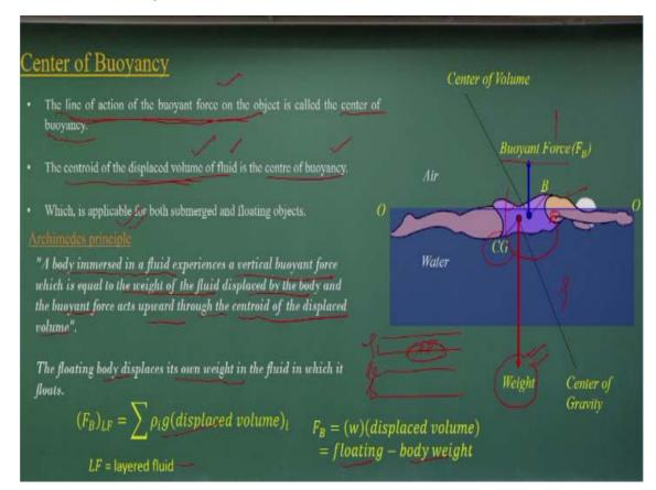
Now if you look it another point is we also look it that the center of buoyancy. That means the line of actions of the buoyant force like we try to compute for the other force component. So line of actions of the buoyant force is the center of buoyancy. That means at which point the buoyancy force acts. That is what the center of buoyancy.
