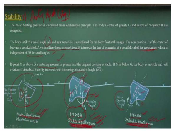
How much stability we have a floating objects. Now let us understand the principles the how the concept is conceived. As we discussed that there will be a gravity force which will act the CG of the floating object and there will be the force which is a buoyant force will act as the CG of the displaced liquid that what will be the center of buoyancy. So these two force components act at two different location.
